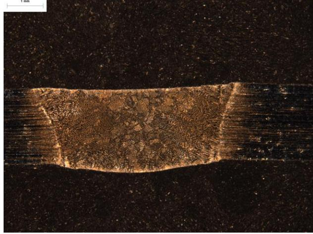
Figure 7.5: Cross-section of full-penetration weld, the current is 56 A, arc length is 4 mm, and welding speed is 1 mm/s
