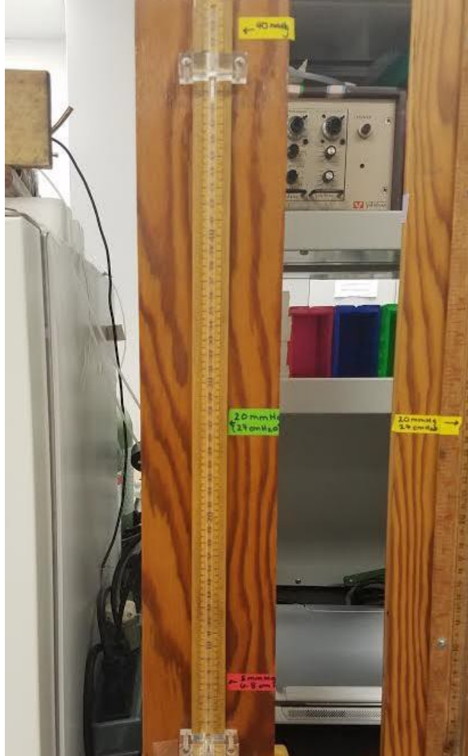
Figure 5: Output monitoring of the pressure system.
