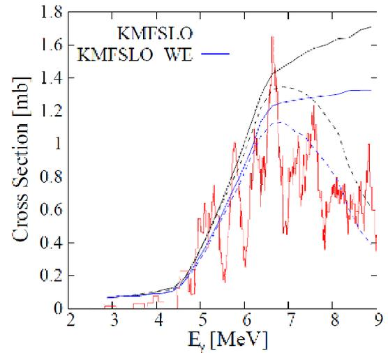
**Figure 3.** Cross sections, integrated over a running window of 250-keV width, for photo-excitation of  $1^-$  states in  $^{76}\text{Se}$  and decay to the ground state from data (red line). The (upper) solid black line shows the result of the statistical calculation considering only the combined KMF/SLO PSF for E1 strength. The (lower) solid blue line includes a Weisskopf estimate for M1 strengths. The respective dashed lines impose the experimental detection limit on the calculations.
