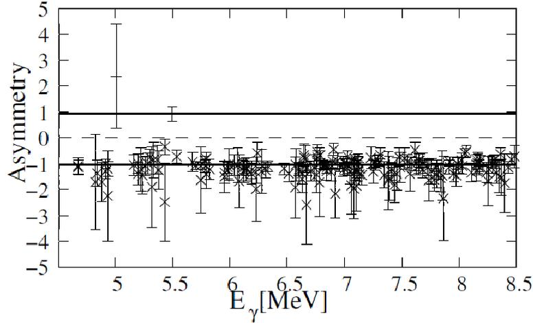
**Figure 1.** Asymmetries ( $A$ ) of ground-state transitions from dipole excited states in  $^{76}\text{Ge}$ . Bars mark the expected limits for positive and negative parity states, the dashed line marks isotropy. E1 (M1) excited negative (positive) parity states have an asymmetry of -1 (+1).
