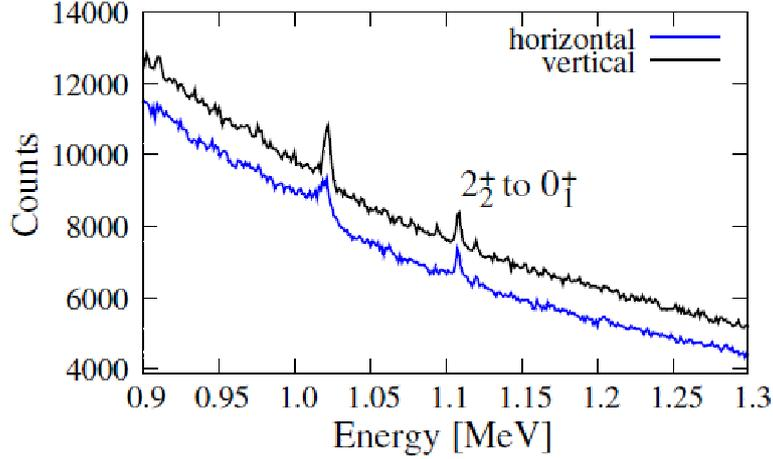
**Figure 2.** A peak from the  $2_2^+ \rightarrow 0_1^+$  transition observed in the horizontal (blue, bottom) and vertical (black, top) detectors, on top of the non-resonant background, far below the beam energy. The peak at 1022 keV stems from  $e^+e^-$  annihilation.
