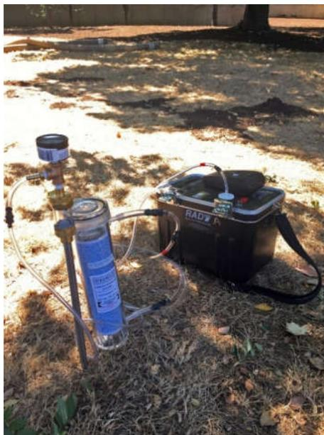
**Figure 1.** RAD7 soil gas testing setup.
