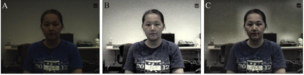
Figure 5.11: Results of histogram equalization for image 2: a) the original image, b) resultant image using GHE, and c) resultant image using CLAHE
