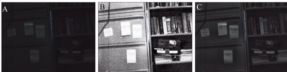
Figure 5.10: Results of histogram equalization for image 1: a) the original image, b) resultant image using GHE, and c) resultant image using CLIAHE
