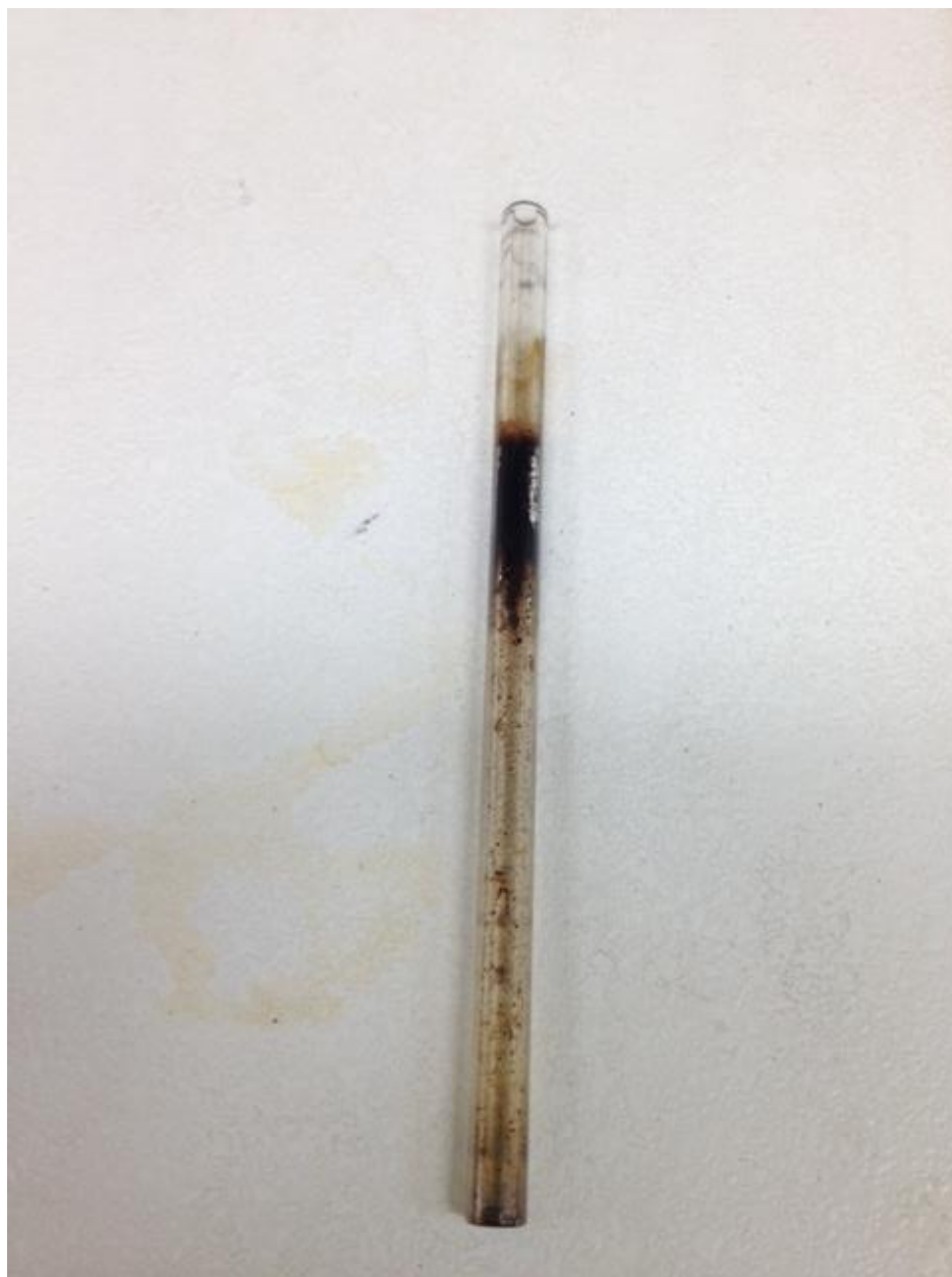
Figure 5.23 GC injector liner after several thioacidolysis samples were analyzed.
