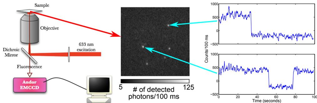
Figure 2. *Left*: Schematic of the experimental set up for single molecule fluorescence spectroscopy. The excitation was 633 nm (532 nm) in the case of Pn-R-F8 (ADT-R-R') derivatives. *Middle*: Image of single molecules of Pn-TCHS-F8 in PMMA. *Right*: Fluorescence time trajectories for the two molecules. The top represents a molecule that photobleaches. The bottom represents a molecule that blinks.
