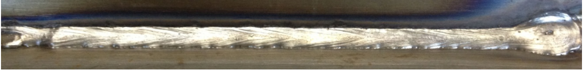
Fig. 4.5 Weld Bead in “Small-Root opening” Experiment (Direction: Right to Left)
