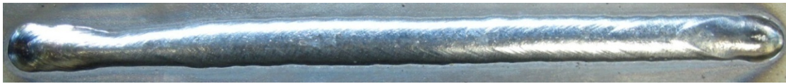
Fig. 7.2 Weld Bead in Bead-On-Plate SAW Experiment. (Direction: L to R; the narrower weld bead was produced before the predictive feedback control starts and shows the need for feedback control)
