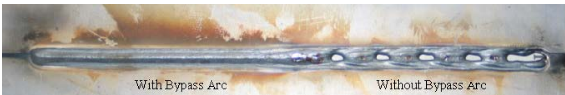
Fig. 2.8 Comparison of weld on lap joint made by controlled DE-GMAW and conventional GMAW process [18]
