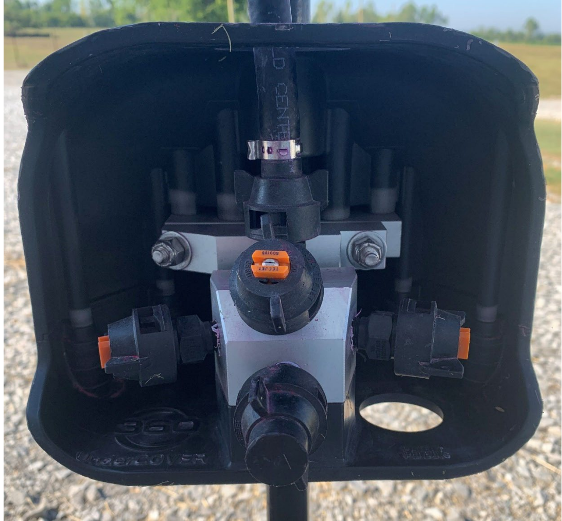
Figure 4-1 Photo of 360 Undercover ® nozzle body (360 Yield, Morton, IL), with a four nozzle arrangement, one horizontally aimed backwards (capped), one horizontally aimed upwards and backwards (Teejet XR8001 tip), and two aimed vertically and outward on each side (Teejet XR8001 tip).
