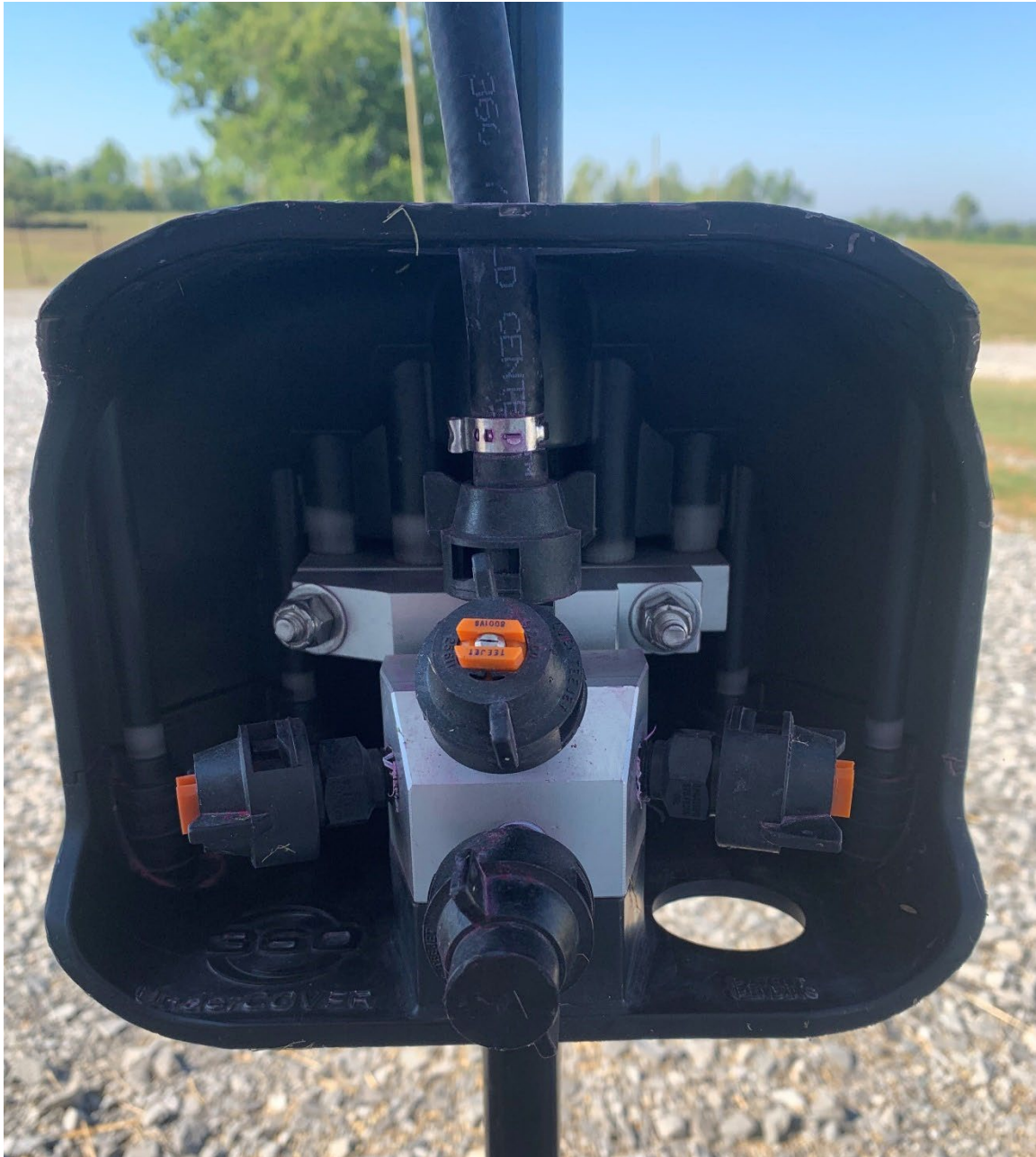
Figure 1-6 A360 Undercover ® nozzle body (360 Yield, Morton, IL) with 4 nozzle arrangements; horizontal and backwards (black cap), horizontal and 45° upwards (orange nozzle tip), and one pointed vertically outward in both directions (orange tips).
