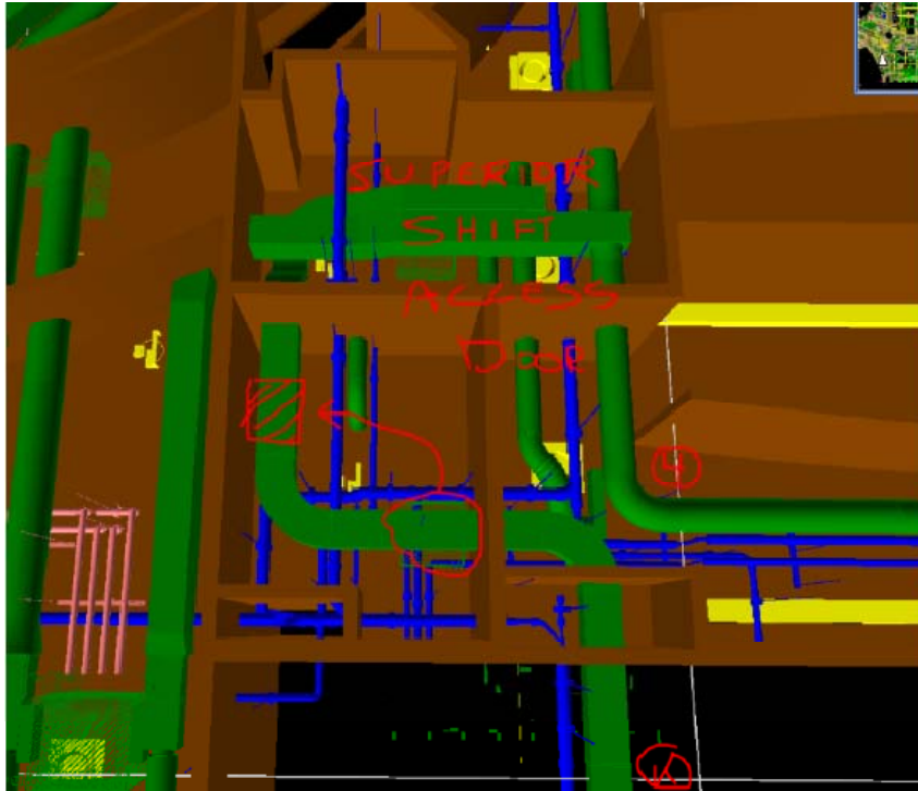
Figure 7.15: Example 2 – Shift Access Door to Avoid Piping
