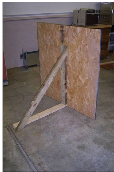
Figure 2. Oriented strand board (OSB) target object (shown from behind so that stand is visible).
