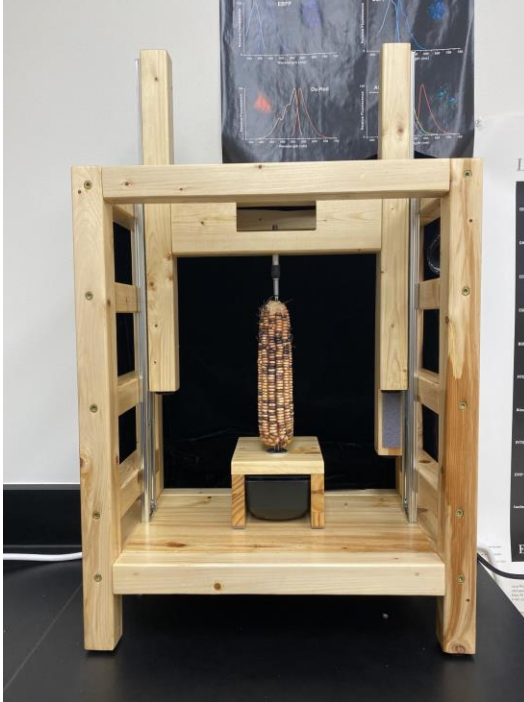
Figure A.6 Maize Ear Phenotyper, developed by Cedar Warman et al. 2021, and modified by Mr. Daniel Murphy. 2D image of an Ornamental Maize Ear, performed using the procedures described in the methodologies.
