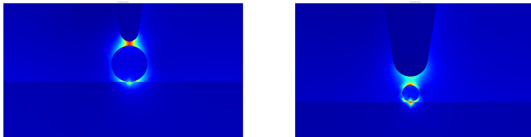
Figure 3.9: Effects of different tip sizes. Left: AuNP diameter 40 nm. Right: AuNP diameter 10 nm. In both cases, the Si tip apex diameter is 20 nm.
