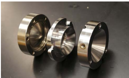
Figure 2.6. Ion trap elements: two end-caps and one ring electrode.
