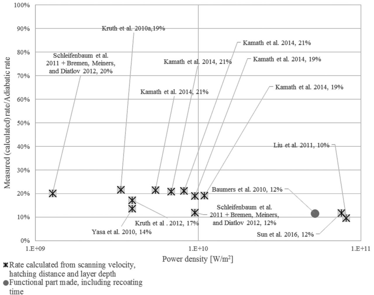
**Figure 2** Measured rate/adiabatic rate (adiabatic efficiency) vs. laser power intensity ( $\text{W}/\text{m}^2$ ) for steel powders for different additive equipment using larger lasers and defocusing.  $\text{W}/\text{m}^2 = \text{watts per square meter}$ .
