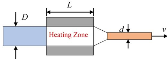
**Figure 4** Heating zone for the plastics extrusion process (sometimes called fused deposition modeling [FDM]). The cylindrical filament enters as a solid with diameter  $D$  on the left, is heated by conduction from the wall in a zone of length  $L$  and exits as a molten polymer of diameter  $d$  and velocity  $v$  on the right.
