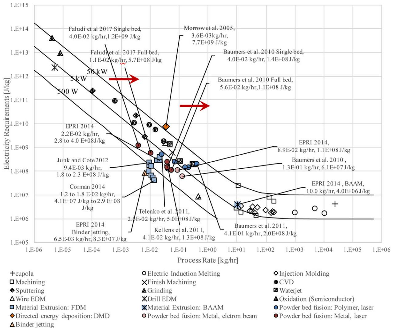
**Figure 1** Energy intensity, J/kg (electricity), and process rates, kg/hr for additive equipment (colored data points) compared to other manufacturing processes. Red symbols indicate additive metals, and blue symbols indicate additive polymers. Note: EDM is electrical discharge machining, FDM is fused deposition modeling, DMD is direct material deposition, BAAM is big area additive manufacturing, and CVD is chemical vapor deposition. J/kg = joules per kilogram; kg/hr = kilograms per hour:
