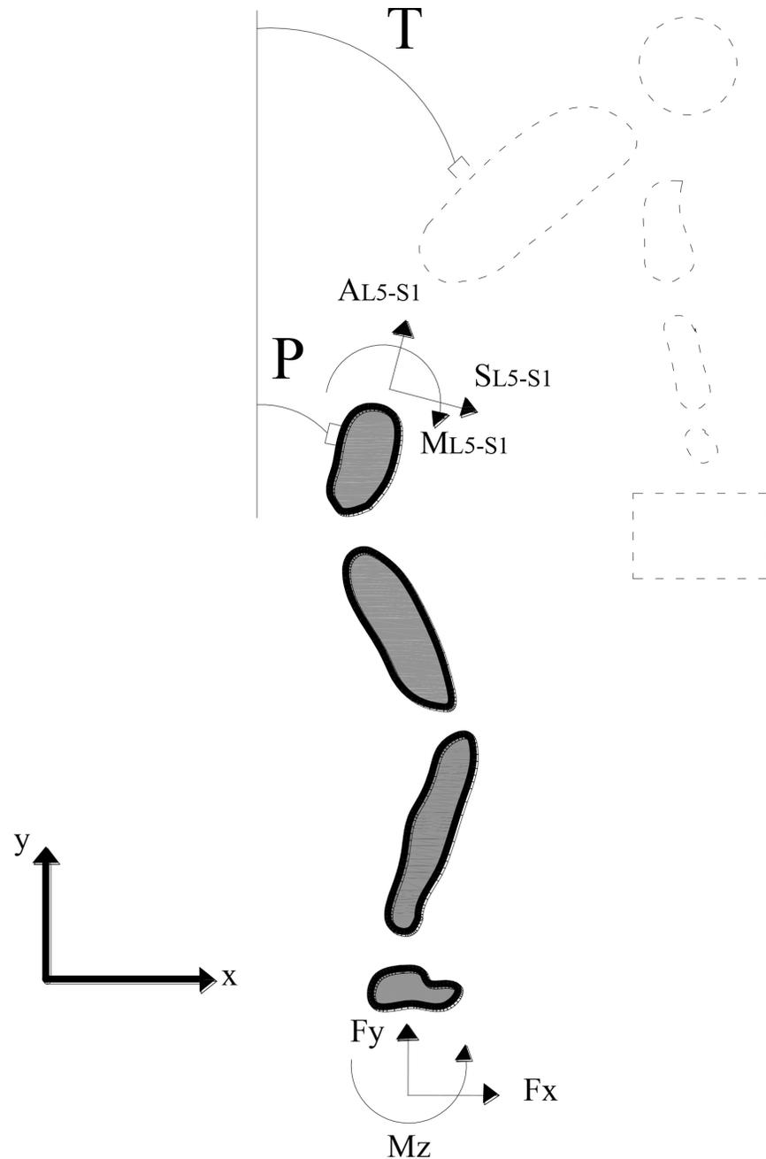
**Figure 1.** Lateral view of the linked-segment model. Pelvic (P) and thoracic (T) rotations are shown in the figure and  $F_x$ ,  $F_y$  and  $M_z$  denote ground reaction forces. Segments with solid lines were included in the “bottom-up” inverse dynamics approach.  $A_{L5-S1}$  (axial),  $S_{L5-S1}$  (shearing), and  $M_{L5-S1}$  (moment) represent the mechanical demands of task on the lower back.
