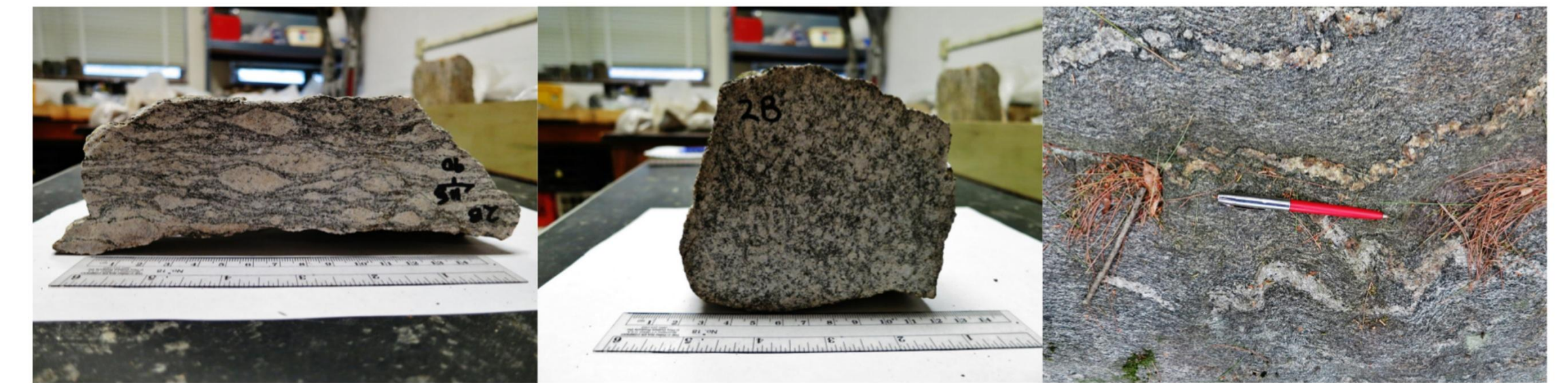
Left: Strongly foliated Hardwick Fm. with feldspar porphyroclasts in a fine grained mica + qtz matrix. Center: Medium grained, undeformed Hardwick Fm. Right: Foliated and refolded Hardwick with folded leucosomes on horizontal face of outcrop next to Carter Rd.
