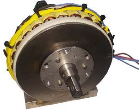
Fig. 10. The ultra high efficiency AFPM machine selected for prototyping based on the comprehensive optimization study with 3D FEA models.
