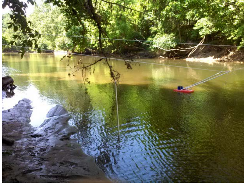
Photograph 3: Using an Acoustic Doppler Current Profiler to collect stream discharge over a tidal cycle.
