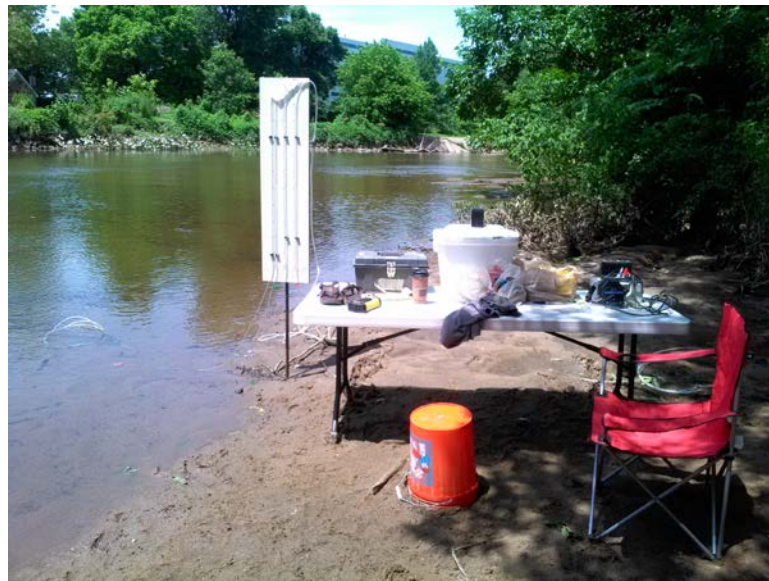
Photograph 2: Sampling of vertical head gradients at low tide using a manometer board.
