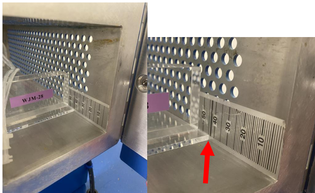
Figure 2.8. Placement of animal holder in high-power focused microwave
