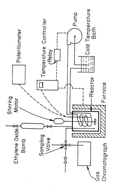
Fig. I. Schematic of Experimental Set-up
