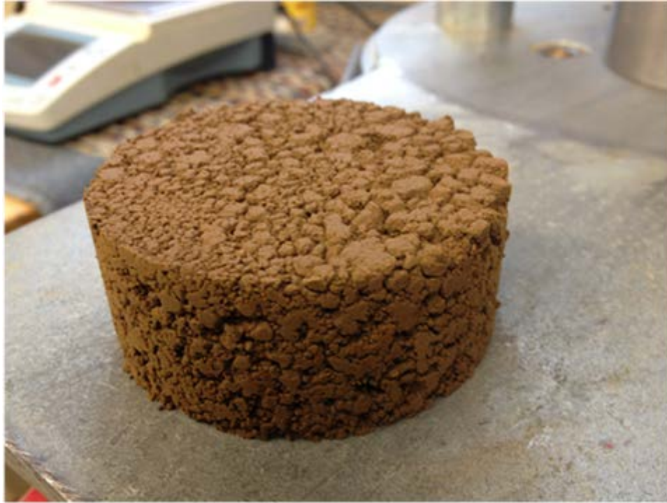
Figure C.9 (a) Shelby tube section containing molded SWCC sample mounted on extrusion piston (b) extruded SWCC specimen.
