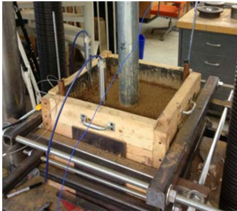
Figure C.40 Shelby tube sampling of the bulk soil.
