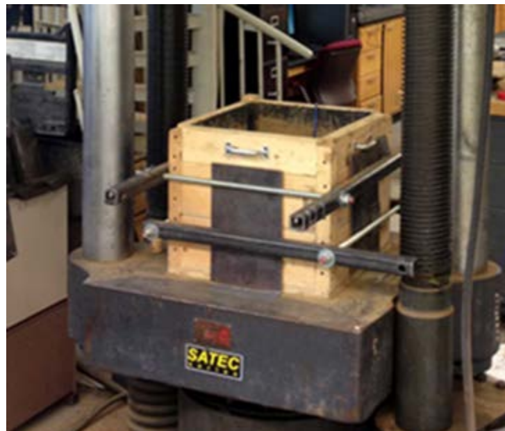
Figure C.31 Bracing of the bulk soil compression containment.
