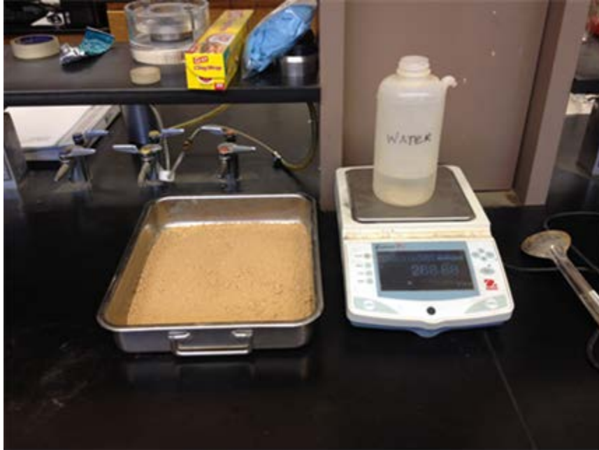
Figure C.8 Soil sample preparation of a batch of oven-dried soil to be mixed with the weighed water to bring the batch sample to the desired moisture content.
