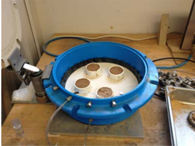
Figure C.15 SWCC pressure chamber with soil samples placed on the ceramic plate.
