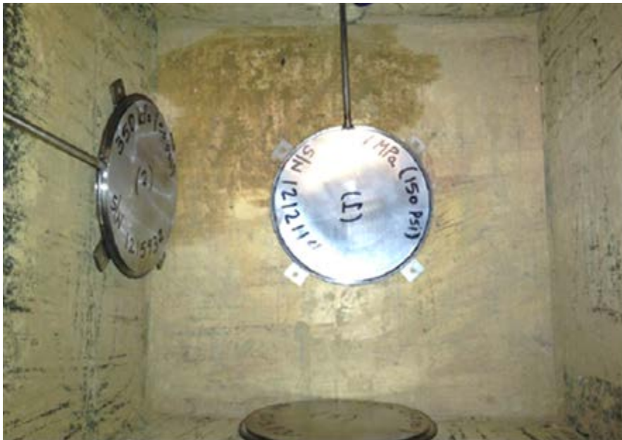
Figure C.32 Earth pressure cell configuration in the bulk soil compression containment apparatus (an overhead view).
