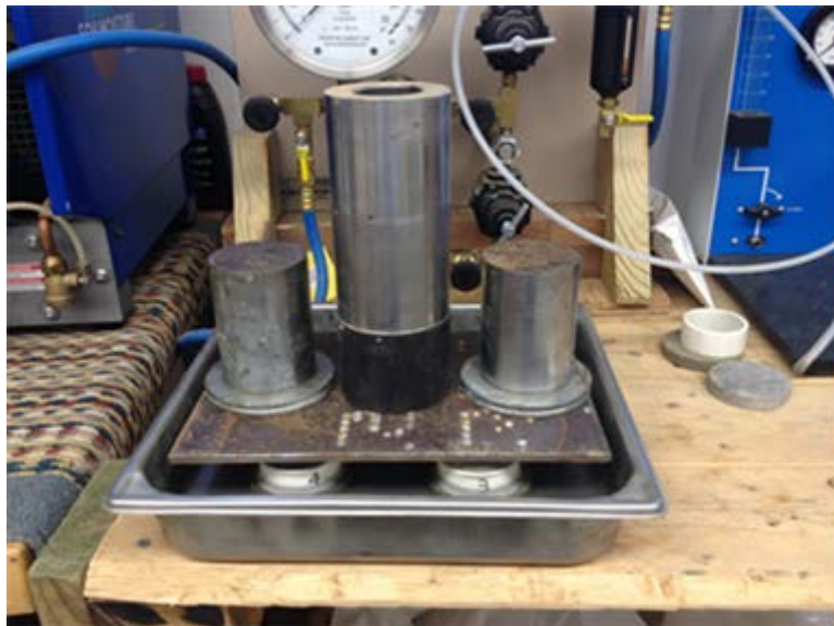
Figure C.12 Weights placed atop porous stones on top of the SWCC specimens for the duration of saturation to stop potential swelling of the specimens.
