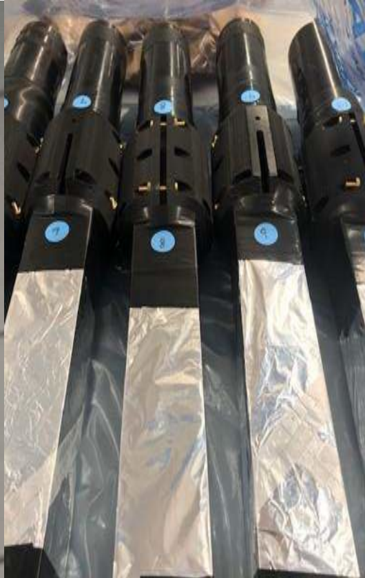
Image 2: Test Bench Data of CsI Detectors and PMTs
