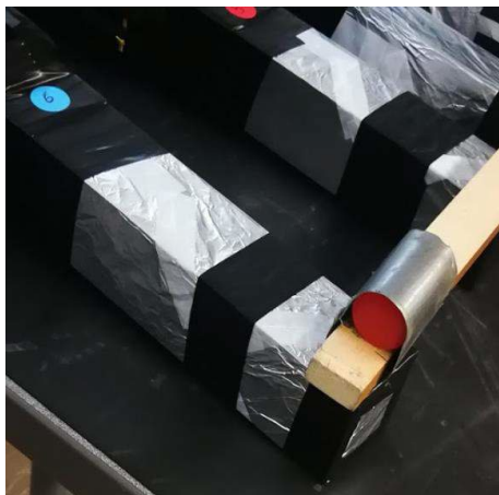
Images 3: Co-60 source on the detectors
