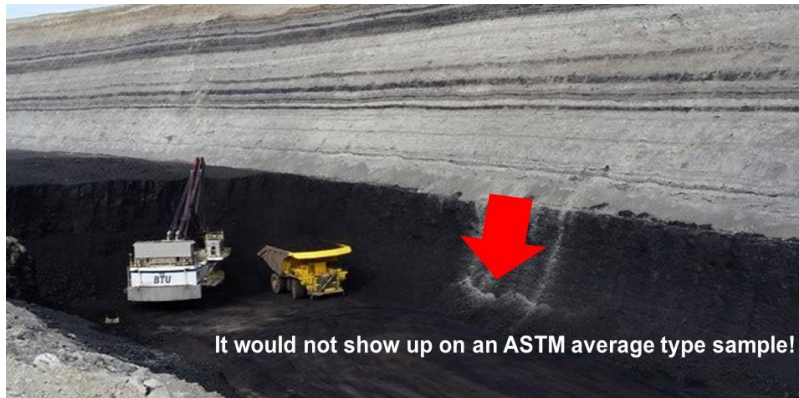
Figure 1. Out of seam dilution visible in coal pit.
