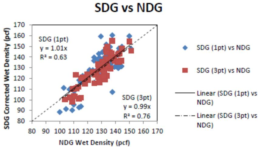
**Figure 2.13: 1-point and 3-point correction results (Rose, 2013)**
