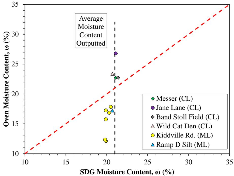
**Figure 4.4: SDG moisture content versus oven moisture content**
