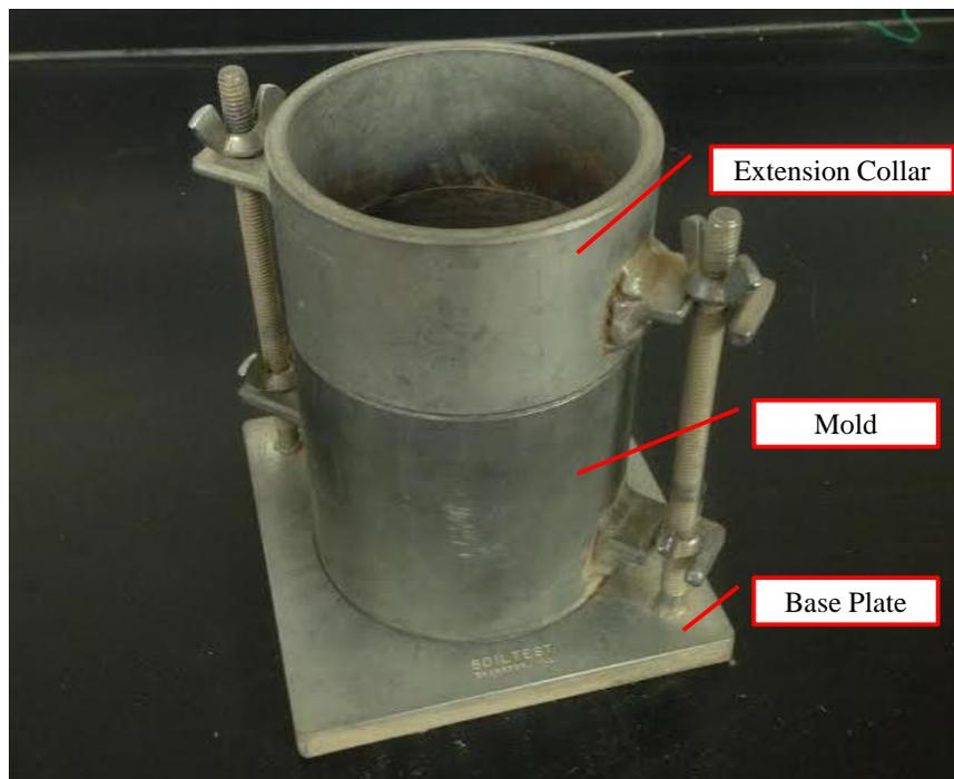
**Figure 3.1: Standard Proctor Mold used for calibrating Soils**
