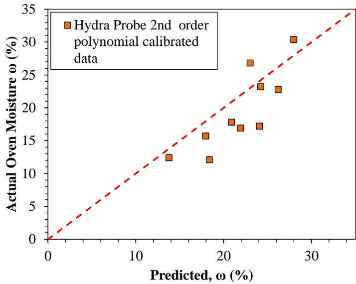
**Figure D.2: Hydra Probe predicted gravimetric moisture content using 2<sup>nd</sup> order polynomial equation**
