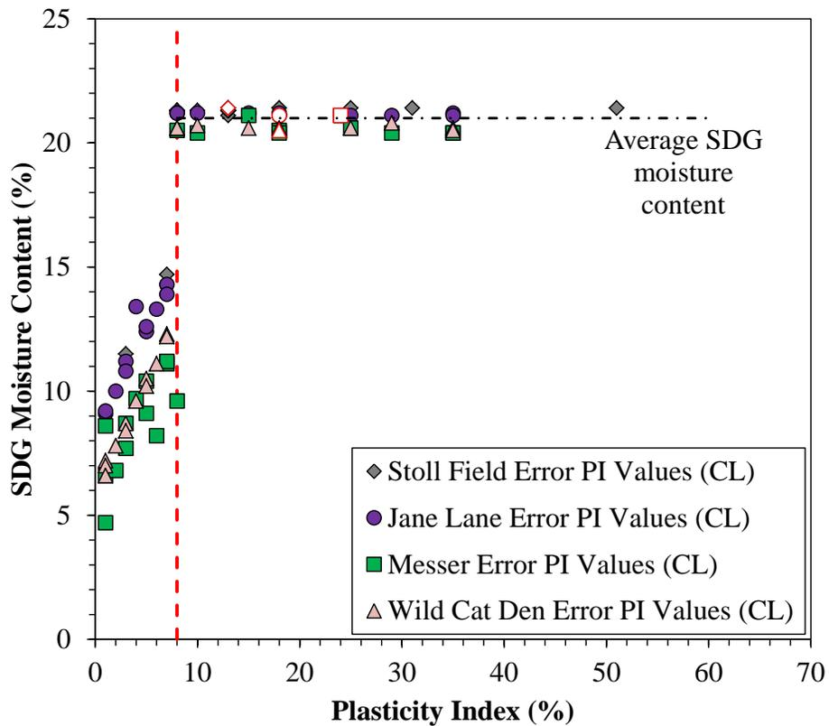
**Figure 4.7: Plasticity index versus outputted SGD moisture content**
