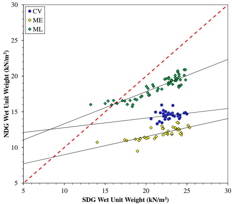
**Figure C.2: Soil-specific trend lines for soil types CV, ME and ML**
