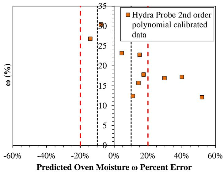
**Figure D.4: Hydra Probe percent error graph of predicted gravimetric moisture content using 2<sup>nd</sup> order polynomial equation**
