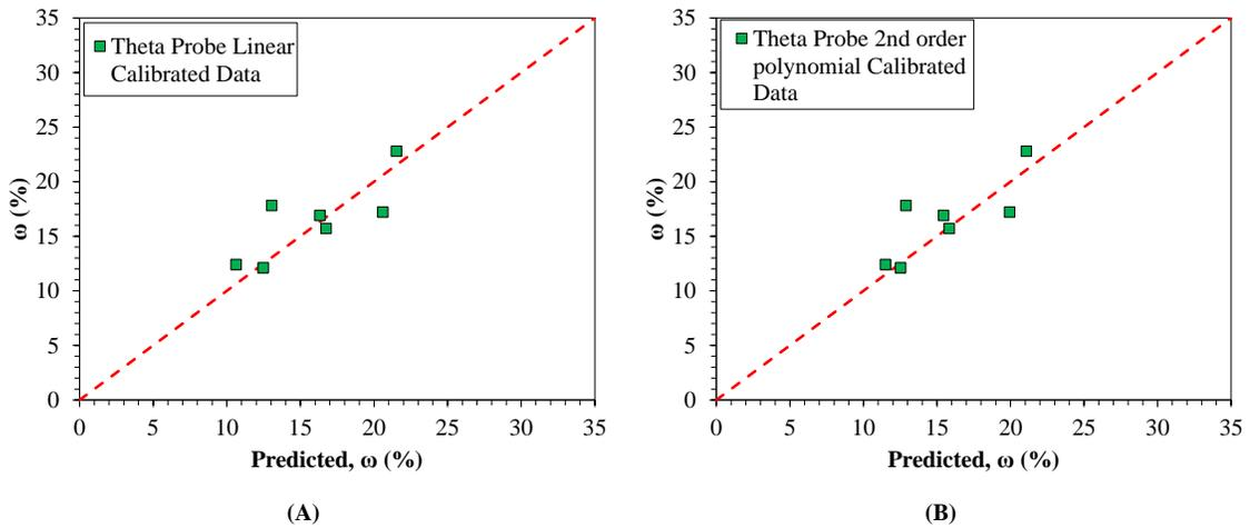
**Figure 6.1: Predicted gravimetric moisture content versus actual gravimetric moisture content; (A) Linear trend line calibrated data; (B) 2<sup>nd</sup> order polynomial trend line calibrated data.**
