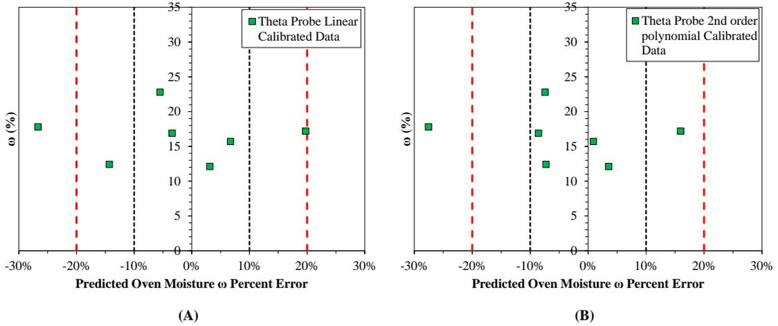
**Figure 6.2: Percent error graphs of predicted versus actual moisture content; (A) Linear calibrated data; (B) 2<sup>nd</sup> order polynomial calibrated data.**
