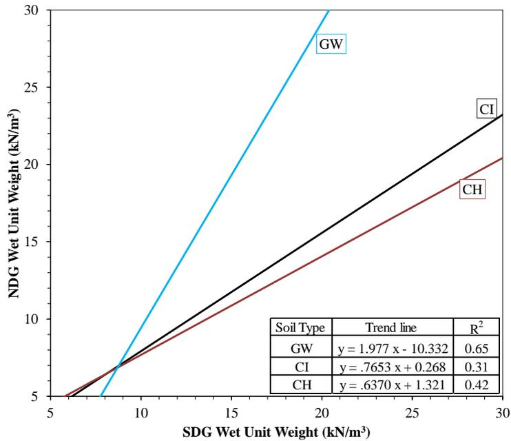
**Figure C.6: Graph to obtain equivalent NDG wet unit weights from SDG wet unit weights; GW, CI, CH**
