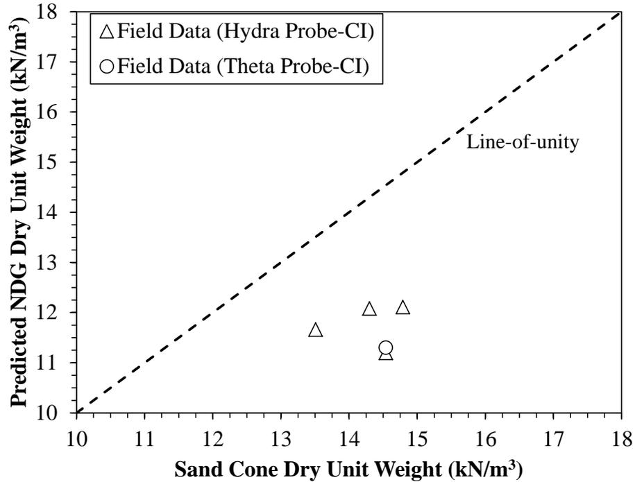
**Figure 6.3: Sand cone dry unit weight compared to predicted NDG dry unit weight**
