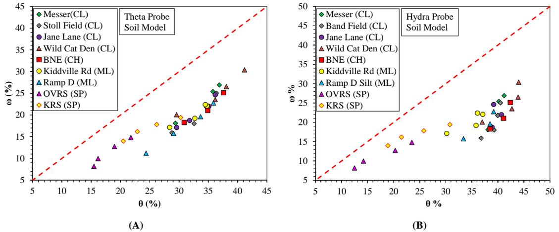
**Figure 3.3: Device Volumetric moisture content vs Gravimetric Oven Moisture Content per soil type; (A) Theta Probe; (B) Hydra Probe.**
