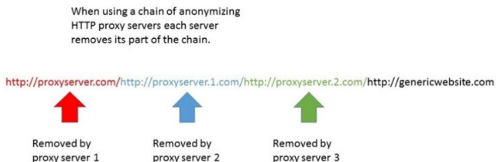
Figure 3. Rewebber chain constructed using three rewebbers
