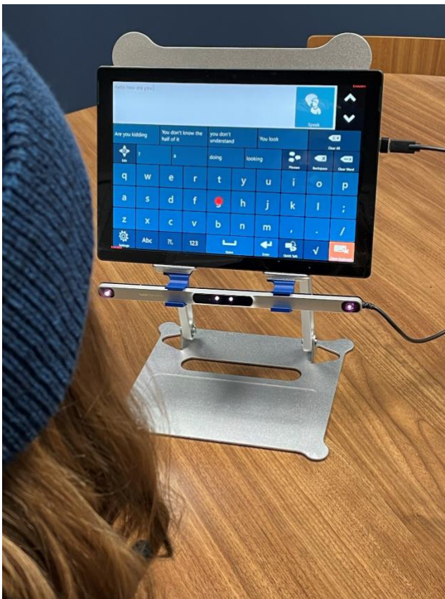
Figure 1.2 High-Tech, Speech-Generating Eye-Gaze AAC System
