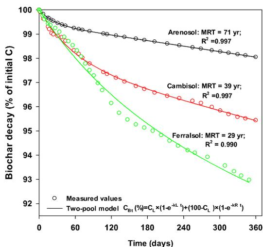
**Fig. 1.** Percent of biochar-C decayed in Arenosol (black), Cambisol (red) and Ferralsol (green) over 12 months. A two-pool exponential (solid line) model was employed to estimate the biochar-C mean residence time.
