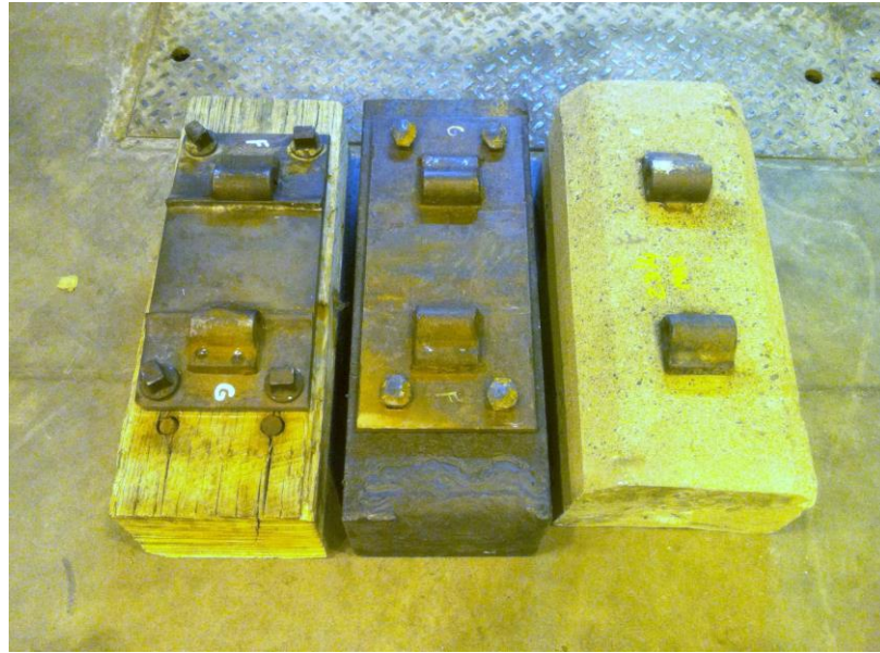
Figure 5.3 Three sections of tie used for laboratory ballast box testing
