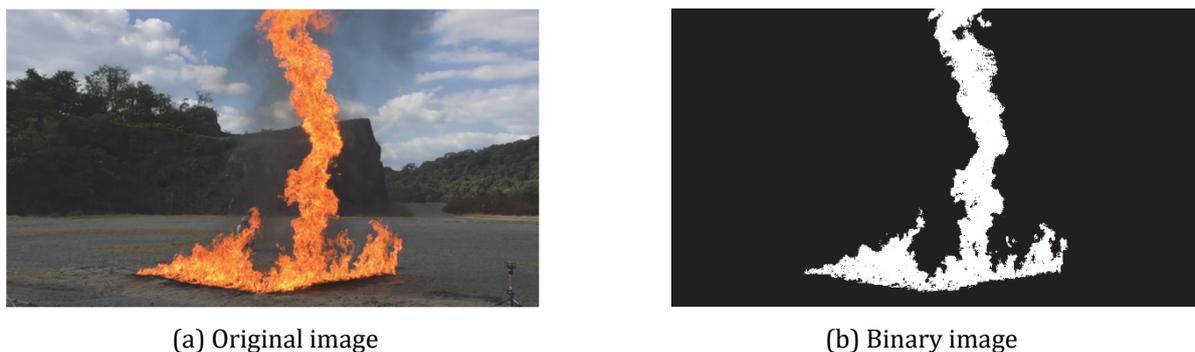
Fig. 3. A typical fire whirl formed in test A.
