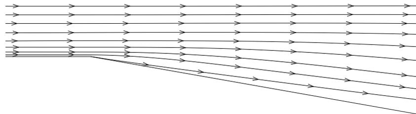
**Figure 17:** Velocity streamlines for the ideal flow analysis.
