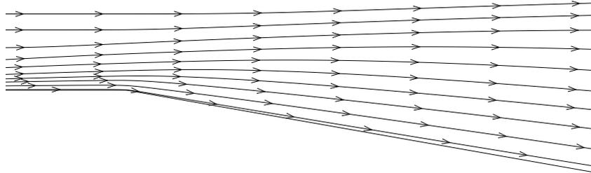
**Figure 15:** Velocity streamlines for the Navier-Stokes analysis.
