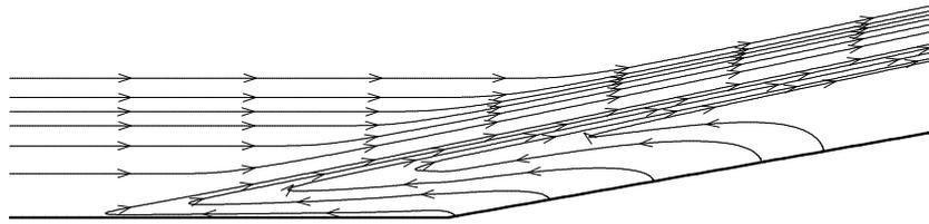
**Figure 7:** Velocity streamlines for the viscous MHD analysis with  $B_y = 0.025$  T.
