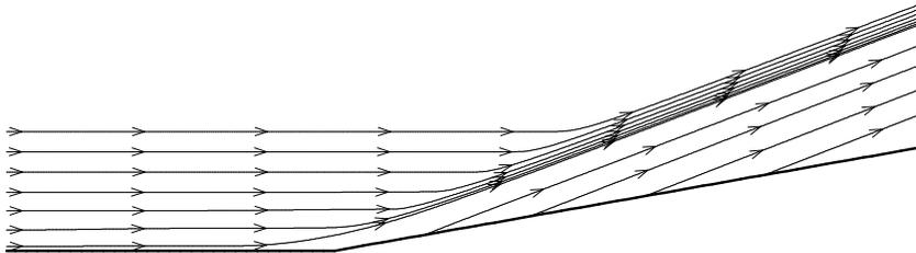
**Figure 9:** Velocity streamlines for the ideal MHD analysis with  $B_y = 0.025$  T.
