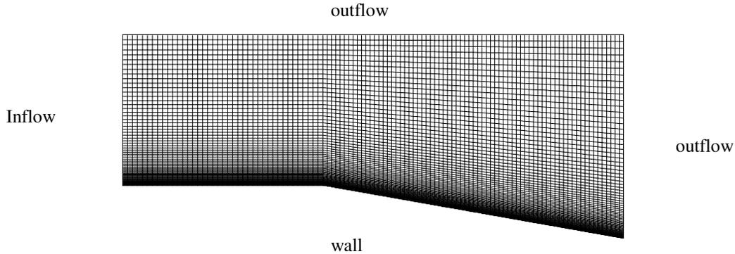
**Figure 10:** Computational grid used for expansion corner analysis.
