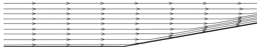
**Figure 8:** Velocity streamlines for the ideal flow analysis.
