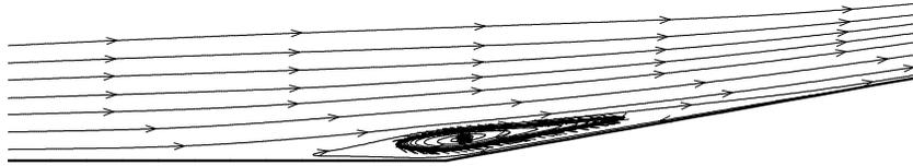
**Figure 6:** Velocity streamlines for the Navier-Stokes analysis.
