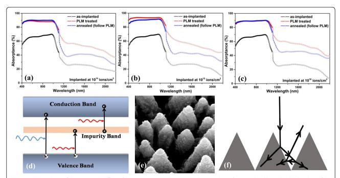
Fig. 1 a-c Dependence of absorptance on different fabrication process with various implantation doses. d Impurity band located within bandgap of Si facilitates generation of carriers which participate in absorption of lower energy photons. e Scanning electron micrograph of silicon spikes. f Illustration of optical path on microstructured surface
