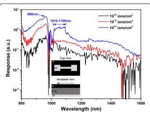
**Fig. 3** Photoresponse of n+/p detectors with different ion-implantation dose. Inset shows the top view and sectional view of the device. Light gray shows the patterns of interdigitated contact on microstructured surface and all standing contact on backside
