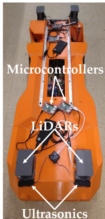
Figure 5. Prototype equipped with LiDAR and ultrasonic sensors.
