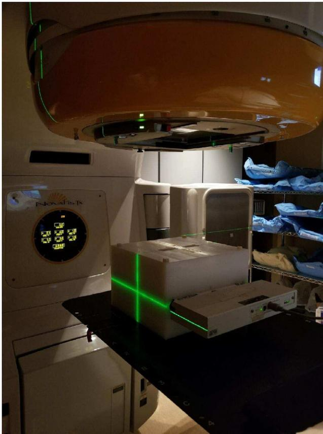
**FIG. 3.** Experimental QA setup in treatment room showing the MapCHECK QA device inserted in the middle of plastic phantom. [Correction added on 8<sup>th</sup> February 2018, after first online publication: Caption was corrected.]
