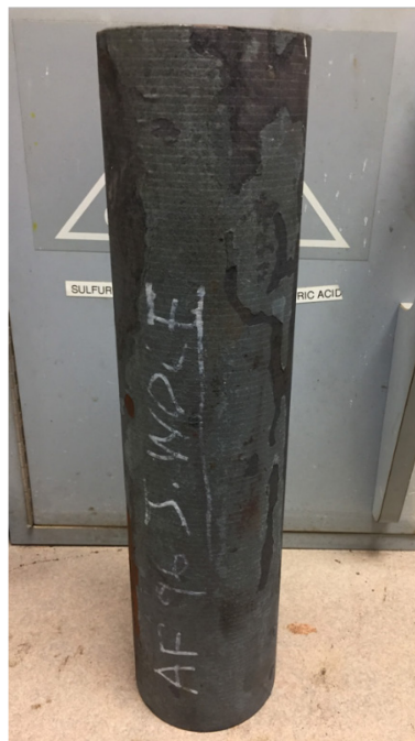
Figure 3-7. Timken-produced AF9628 bar after heat treatment
