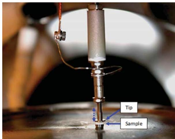
Fig. 1. (Color online) UHV Kelvin probe showing the tip and sample configuration. The probe tip vibrates vertically above the sample. The sample must be grounded with respect to the tip and remain free of any vibration.
