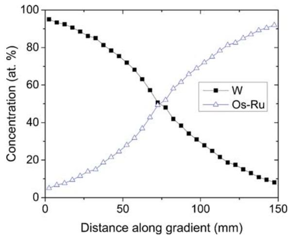
FIG. 2. (Color online) Concentration gradient of W–Os–Ru ternary alloy films deposited on Mo–Re and porous W substrates. The composition for every sample was determined using XPS and select samples were measured with EDS as a cross-check, which gave similar compositions.
