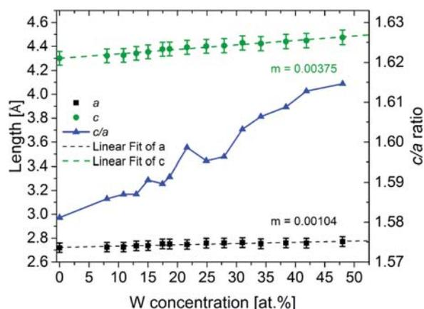
FIG. 4. (Color online) Comparison of variations in  $c$  and  $a$  lattice parameters with  $W$  concentration. The variation in  $c/a$  ratio is also shown plotted against the right axis. The  $c$  lattice parameter increases over 3.5 times faster than the  $a$  lattice parameter, indicating that the unit cell expands primarily along the  $c$  axis as  $W$  is added to the HCP Os–Ru phase.
