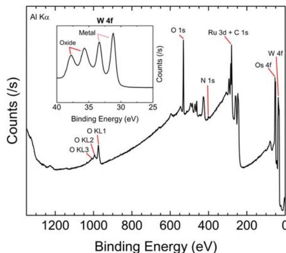
FIG. 7. (Color online) XPS spectrum of W–Os–Ru (51 at. % W) in the as-deposited state. The inset region for W 4f peaks indicates that the alloy surface is partially oxidized. All peaks for major species are labeled. Other peaks can be attributed to core levels of W, Os, or Ru. Additional W–Os–Ru alloy compositions yielded similar spectra.
