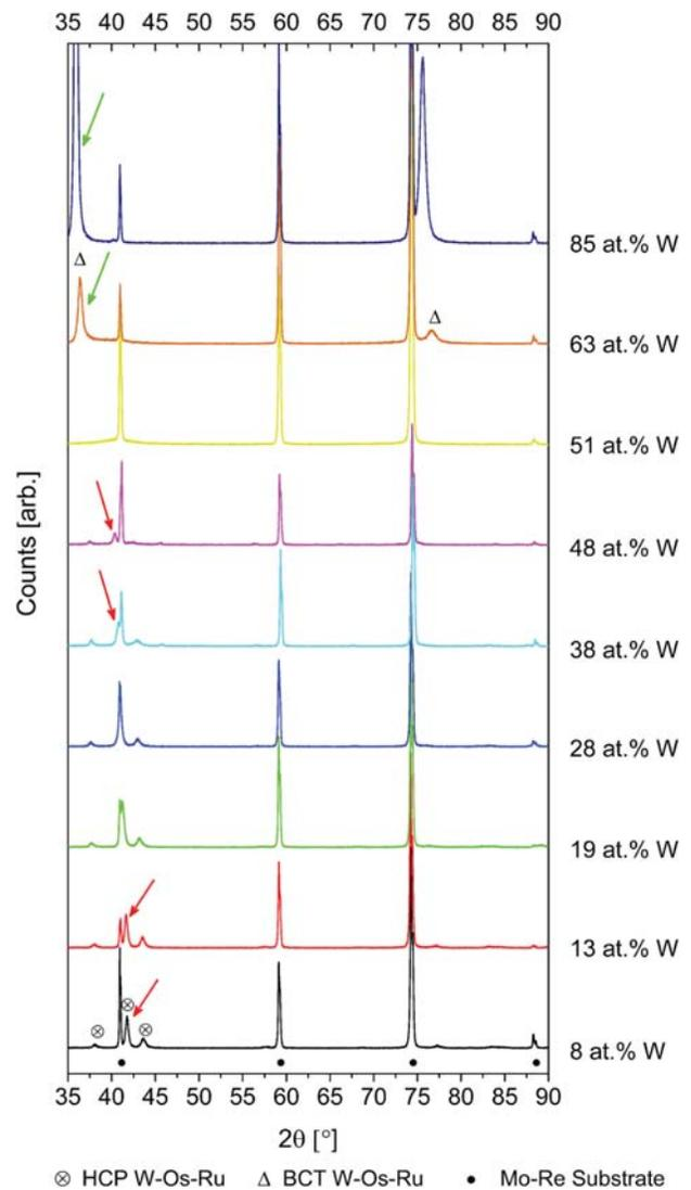
FIG. 3. (Color online) XRD scans of W–Os–Ru ternary alloys indicating a shift in the HCP peak position with increasing W concentration (starting from the bottom, peaks indicated by arrows) and showing the formation of a BCT phase (arrows above the top two XRD scans).
