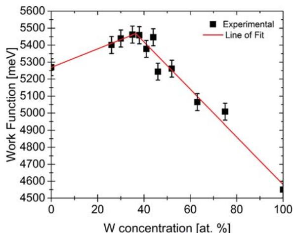
FIG. 6. (Color online) Work function trend of W–Ir alloys with respect to W concentration. There is a peak in the work function at approximately 40 at. % W. This is similar to the peak observed in the W–Os–Ru system, albeit at a slightly higher W content and with a higher value of work function.
