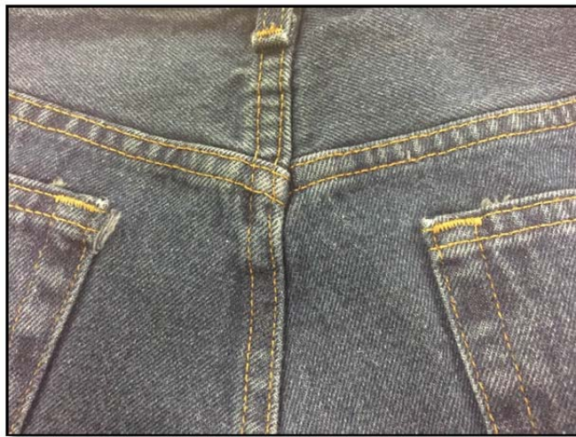
Figure 4.8. Uneven back yoke in Faded Glory jeans
