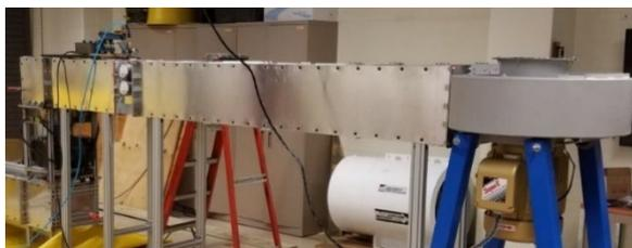
Fig. 7. The experimental set-up to generate the flow-pressure drop curve.
