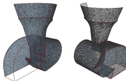
Fig. 4. Polyhedral mesh on the Vortecone surface.
