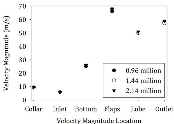
Fig. 5. Plots of velocity magnitudes using three different meshes at the selected points.
