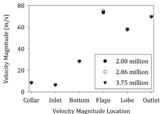
Fig. 6. Velocity magnitudes at the six points full scale Vortecone.
