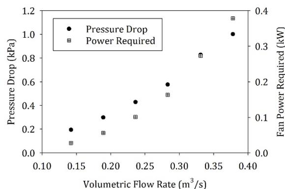
Fig. 9. Projected pressure drop and fan power requirement for the smaller Vortecone.
