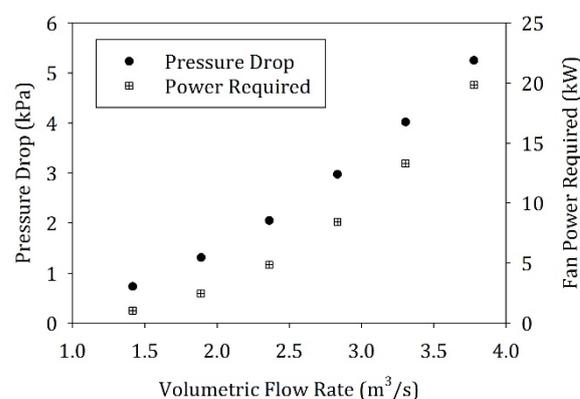
Fig. 10. Projected pressure drop and fan power requirement for a large Vortecone.
