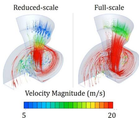
Fig. 11. Streamlines of airflow in the reduced and full-scale model.
