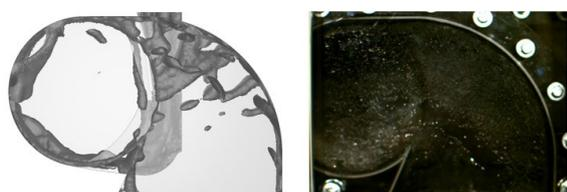
Fig. 13. Comparison of multi-phase CFD model and an image from a high-speed camera during experiments.
