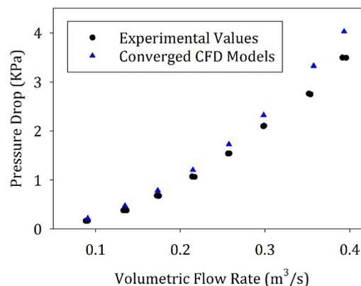
Fig. 8. Pressure drop comparison between CFD models and experimental results.
