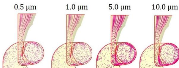
Fig. 2. The trajectory of aerosol particles of different sizes inside the Vortecone.
