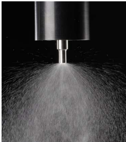
Figure 3-3: This picture shows how the spray droplets are broken up from the bulk liquid solution. Picture courtesy of Sonaer Ultrasonics
