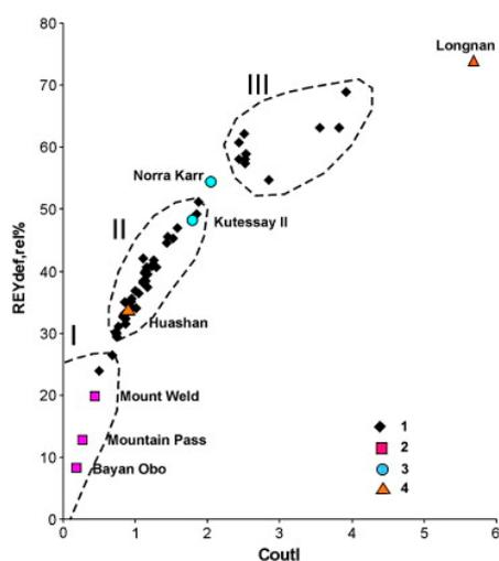
**Figure 2.** Classification of REY-rich coal ashes by outlook for individual REY composition in comparison with selected deposits of conventional types. 1, REE-rich coal ashes; 2, carbonatite deposits; 3, hydrothermal deposits; and 4, weathered crust elution-deposited (ion-adsorbed) deposits. Clusters of REE-rich coal ashes distinguished by outlook for REY composition (numerals in figure): I, unpromising; II, promising; and III, highly promising. From Seredin and Dai [9].
