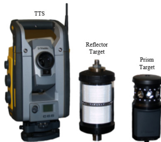
Figure 3. TTS, reflector target, and prism target.
