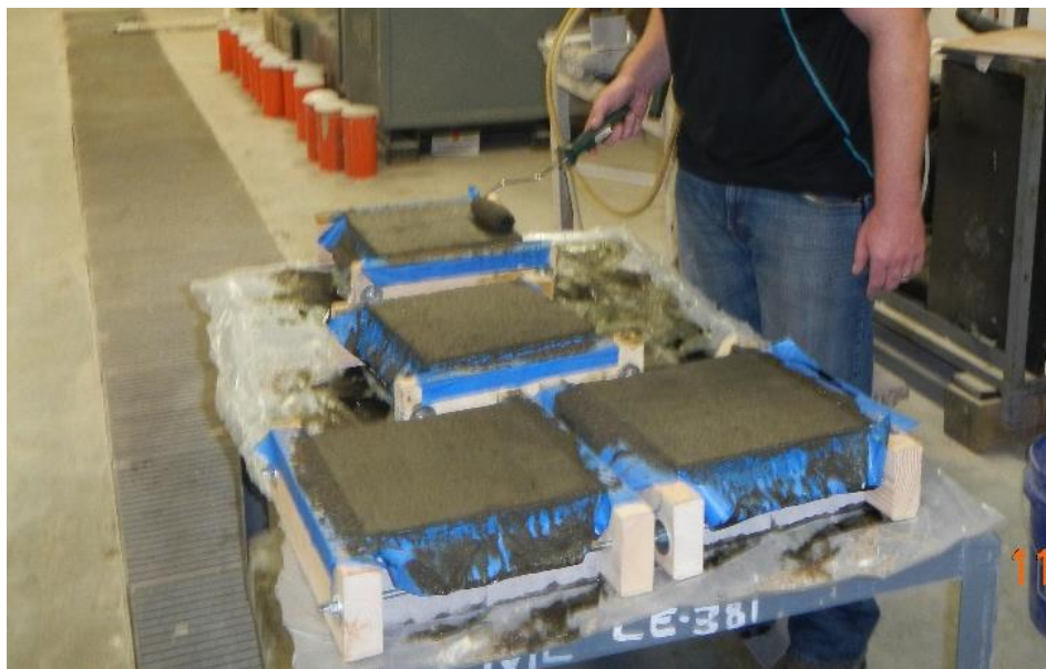
Figure 8 Back-rolling Healer/Sealer Specimens After Application of Sand
