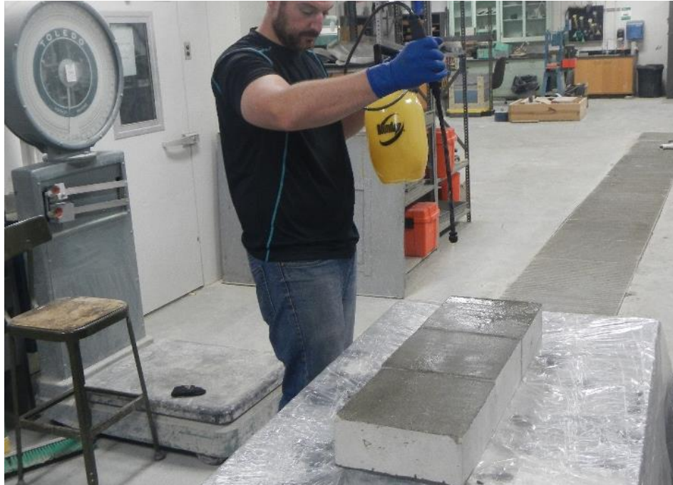
Figure 6 Application of Penetrating Sealer
