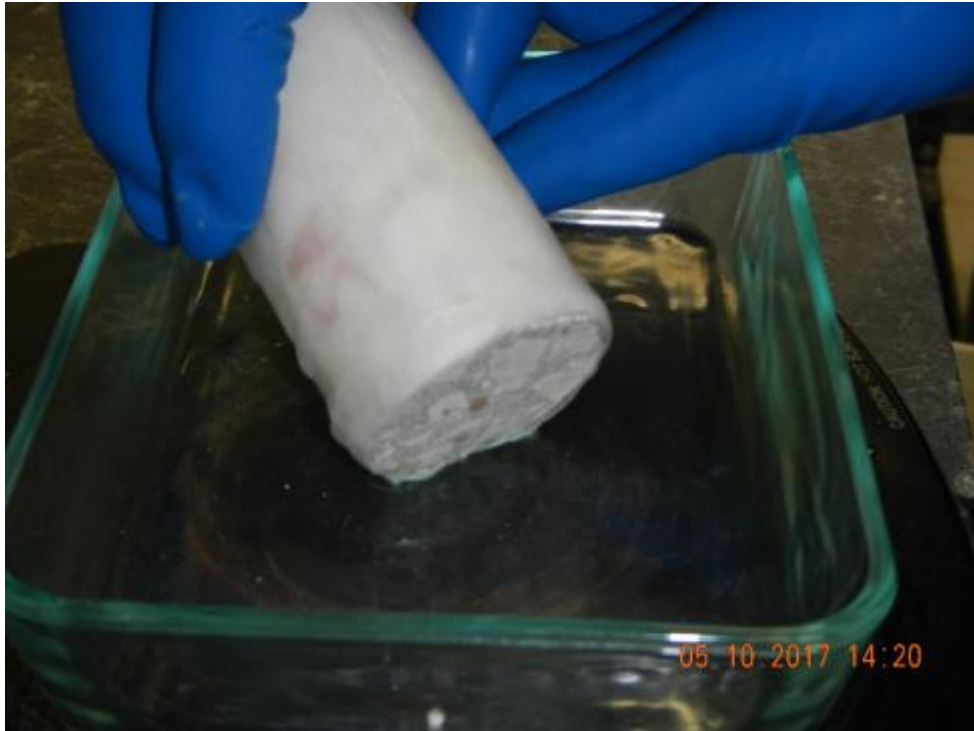
Figure 15 Application of Paraffin to Edges
