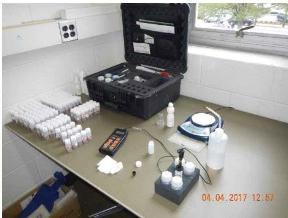
Figure 13 Germann Rapid Chloride Test (RCT)
