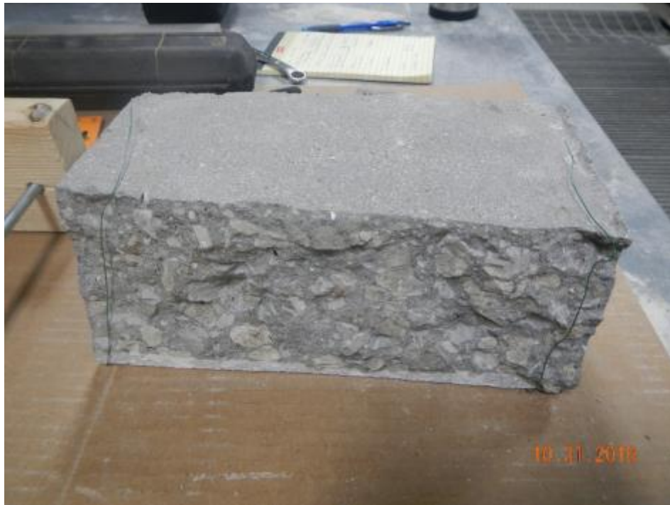
Figure 3 Fractured Surface with Wire Spacer
