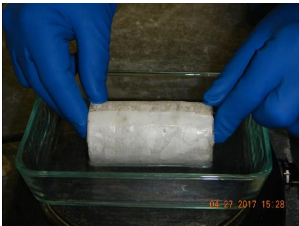
Figure 14 Application of Paraffin with Ends Taped
