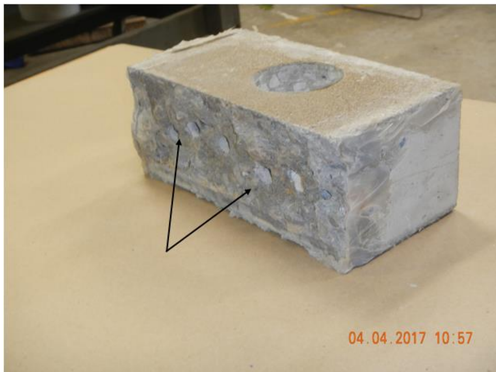
Figure 12 Fractured Surface (Arrows Indicate Sample Collection Area)
