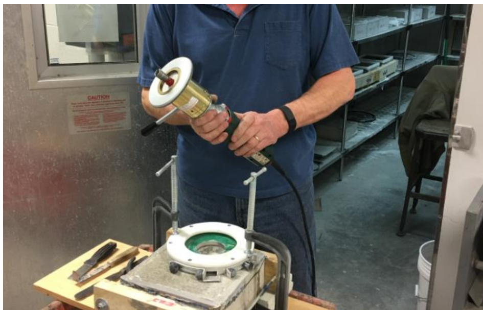
Figure 10 Germann Profile Grinder
