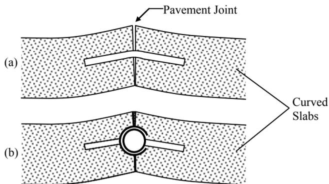
**Fig. 3.** Curling of the Concrete Pavement Slabs with a) Conventional Dowel Bars, and b) Hinged Dowel System.
