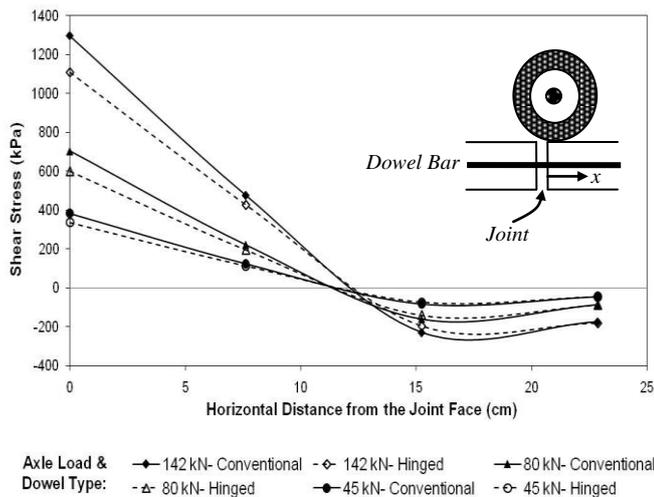
**Fig. 6.** Variation of the Shear Stress Along the Critical Dowel Bar.
