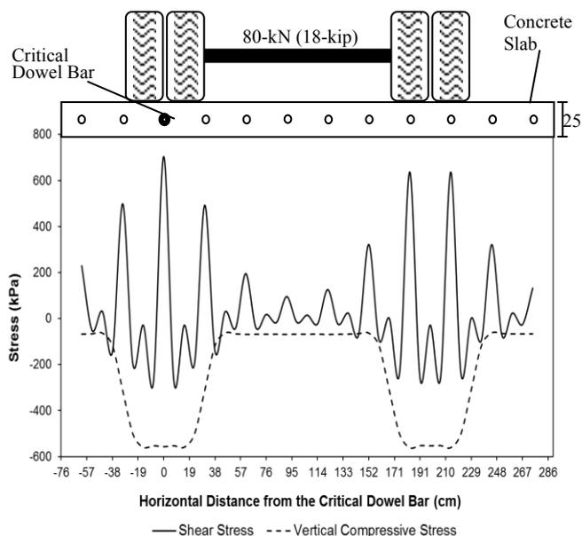
**Fig. 5.** Variation of Shear and Compressive Stresses in a Slab Joint with Conventional Dowel Bars.
