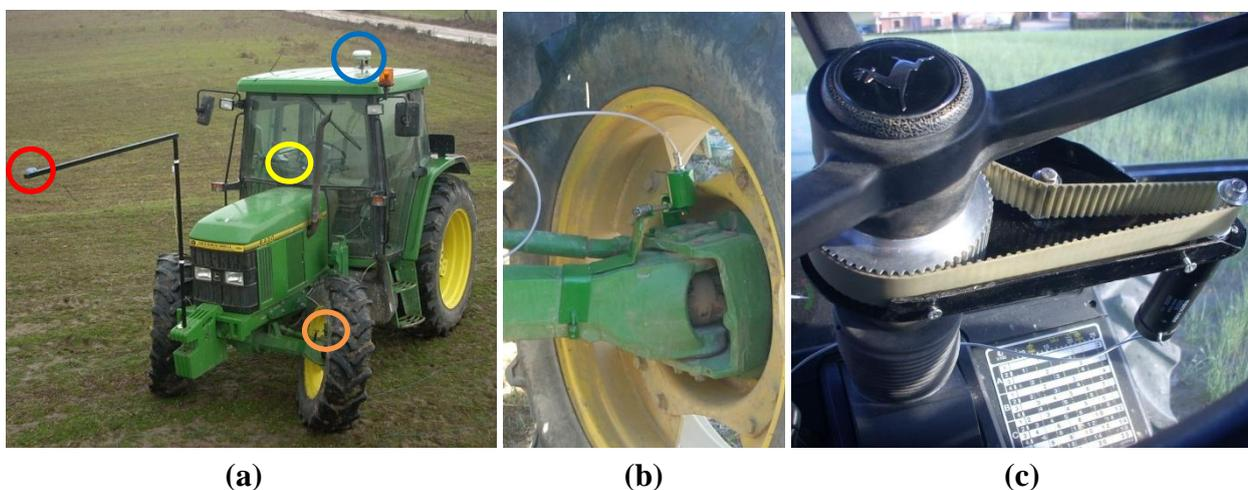
**Figure 6.** Different positions of the Haicom HI-204III navigation GPS in the field tests. The navigation sensor position is highlighted with a red circle. (a) The guidance GPS placed in the back part of the cabin over the rear axle. (b) The guidance GPS placed 3 m ahead of the rear axle of the tractor. (c) The guidance GPS placed 5 m ahead of the rear axle of the tractor.
