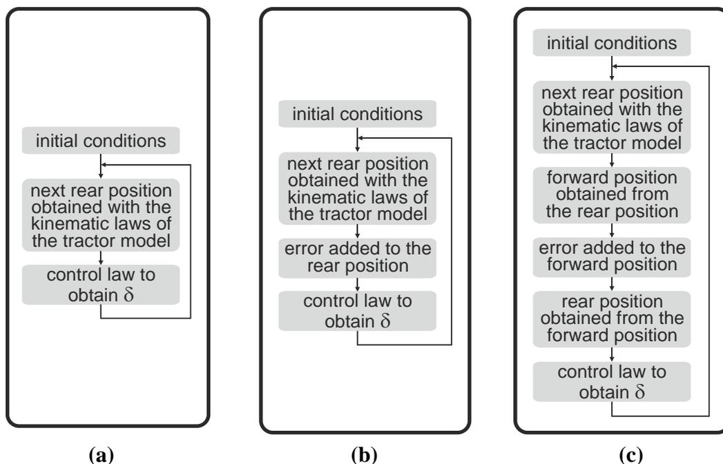
In these simulations, the kinematic model of the tractor presented in Equation (2) and the control law of Equation (14) were employed. The simulation rate was 1 Hz. Constants  $L = 2.3$  m,  $u = 1$  m/s, and the control gains obtained experimentally in the field test ( $k_1 = 0.08$ ,  $k_2 = 0.5$ ) were fixed. Experimental errors of Figure 4 were added to each analytically calculated position of the tractor,
