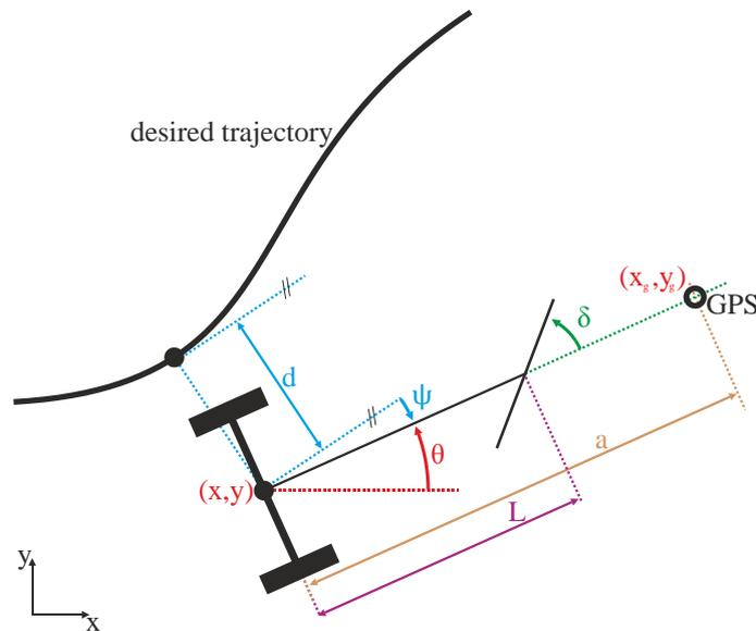
Assuming no-slip conditions on the wheels, the kinematic model of the vehicle is given by:
