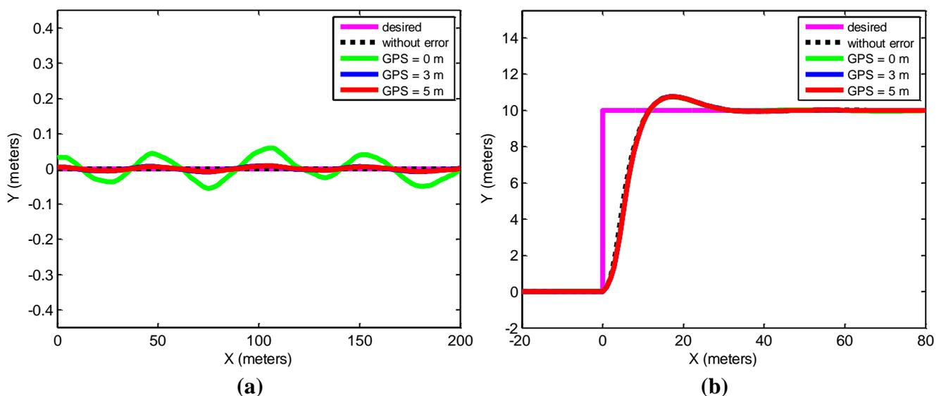
Simulations with different forward GPS guidance positions were performed in order to compute the mean and Root Mean Square (RMS) values of the error. Simulation time was 14 minutes ( $14 \times 60 = 840$  points) and the reference trajectory was a straight line. Table 1 shows the obtained results.
