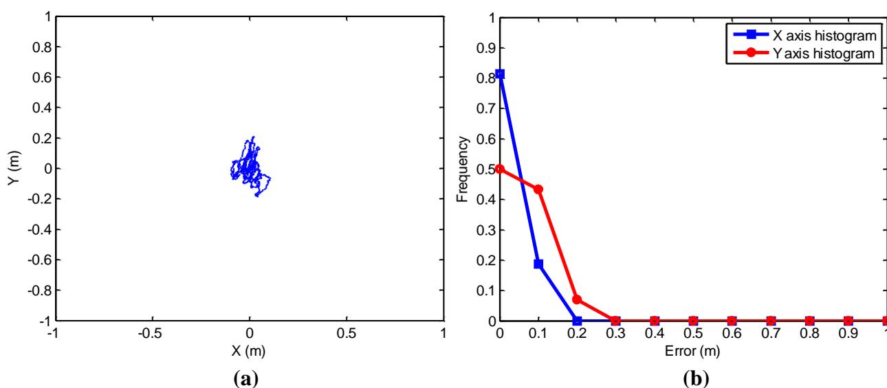
Taking the previous data into account, a low cost Haicom HI-204III GPS receiver can technically be used to guide a tractor when the time between passes is short and precision is not required. The distance between passes could differ by large amounts from the desired when a long time between passes occurs.
