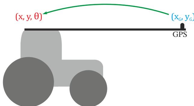
The tractor position  $(x, y, \theta)$  at the midpoint rear wheel axle can be obtained from the positions obtained from the GPS receiver  $(x_g, y_g)$ , either with the kinematic tractor model or from geometric relations.
