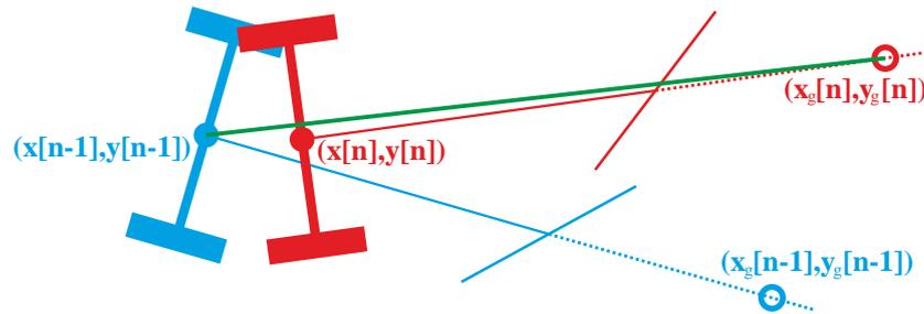
Equation (11) is obtained if it is assumed that  $(x[n], y[n])$  lies along the straight green line that joins  $(x[n-1], y[n-1])$  with  $(x_g[n], y_g[n])$  in Figure 3. Once  $\theta$  is approximately calculated,  $x[n]$  and  $y[n]$  may be obtained with Equations (12) and (13):
