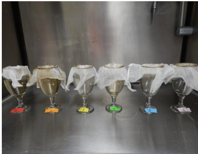
Figure S2. Setup of Baermann apparatus. Picture courtesy of Holli Gravatte.
