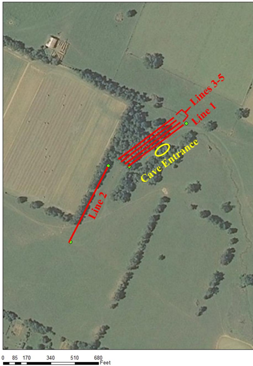
Figure 3.2. Slack's Cave electrical-resistivity survey line locations. Line 5 is at the top of the parallel survey section with (in order) lines 4, 3, and 1 below.
