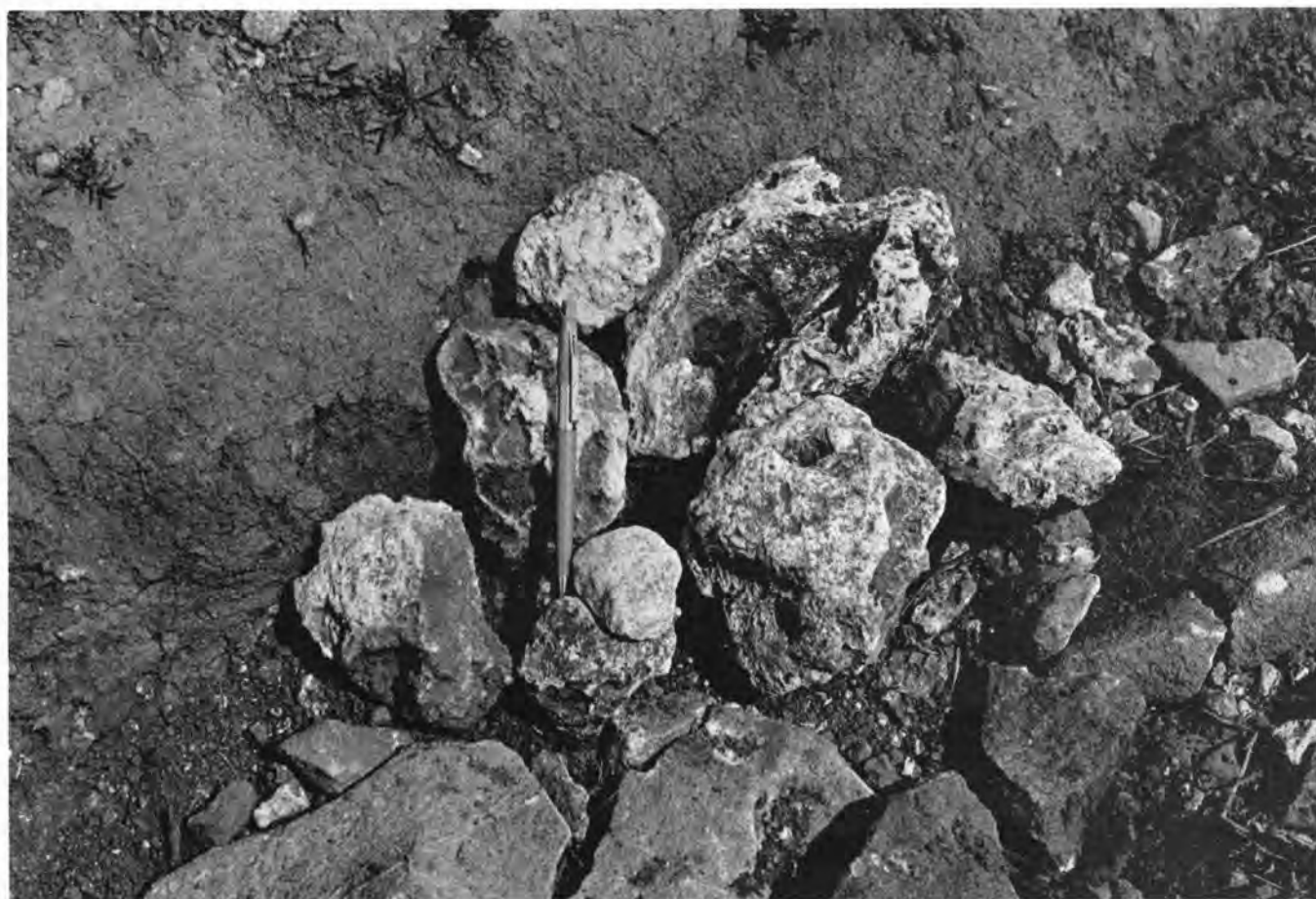
Figure 10. Barite float marks the trace of the Kentucky 590 (Engleman) Vein, Lincoln County.
