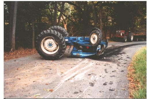
close to the edge of the embankment, the right front wheel dropped over the embankment and the tractor overturned onto the road pinning the victim underneath. The farmer had recently purchased the tractor without a ROPS or seat belt and had overturned the tractor five weeks before, but was able to jump away.
