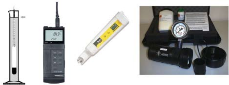
Figure 3. Hydrometer, conductivity meter, conductivity pen, and Agros® N meter (instruments shown are in different scales).
