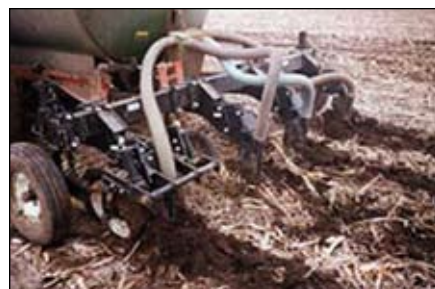
Figure 4. Application and incorporation of manure into soil.
