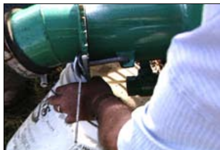
Figure 1. Sampling manure directly from the pumping line.
