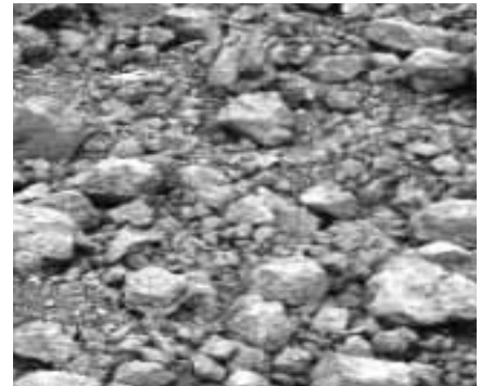
Figure 8. Soil with medium workability is difficult to crumble.
